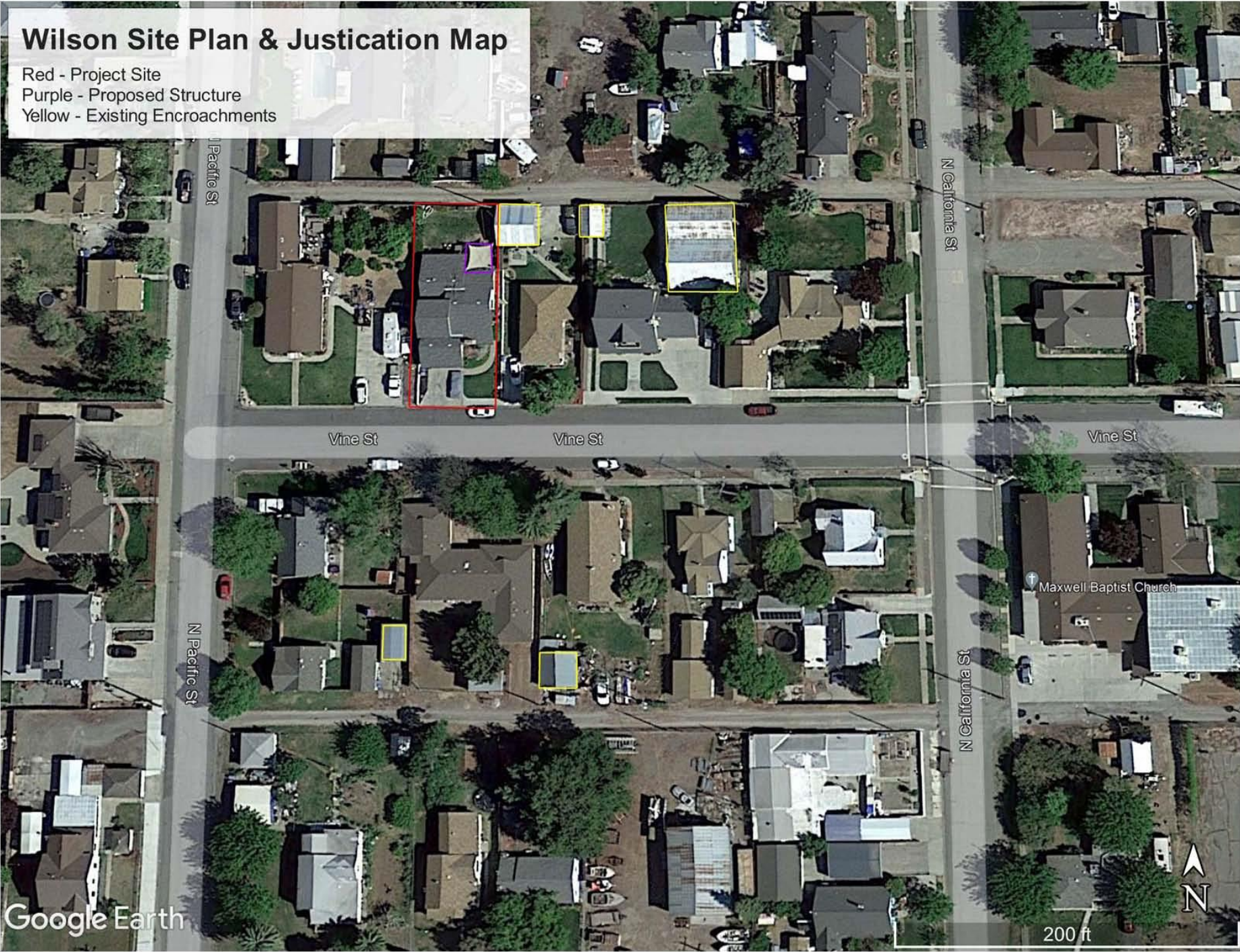
Project Location and Justification Map for the proposed Cheney (Wilson) Variance PD-21-31 reducing the residential accessory building side yard setback from 3 feet to 0 feet t to allow the construction of a 15 feet by 22 feet or 330 square foot patio/deck cover.
