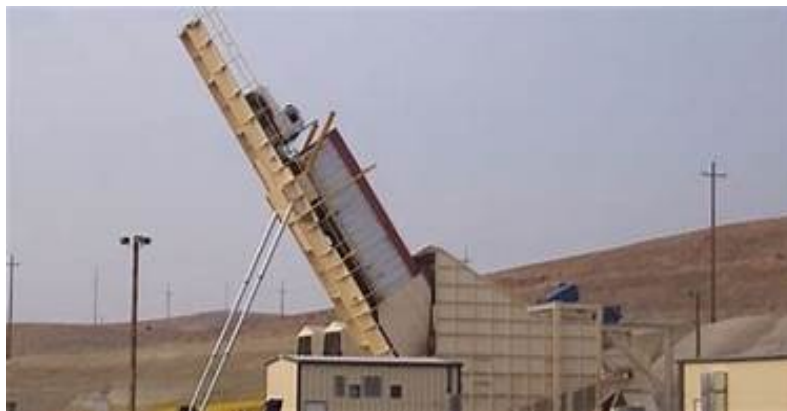
Exhibit 2 Example Hydraulic Truck Dump
