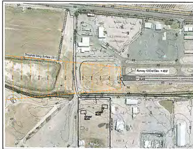
THRESHOLD SIGHTING SURFACE (20:1) 1"=200'
