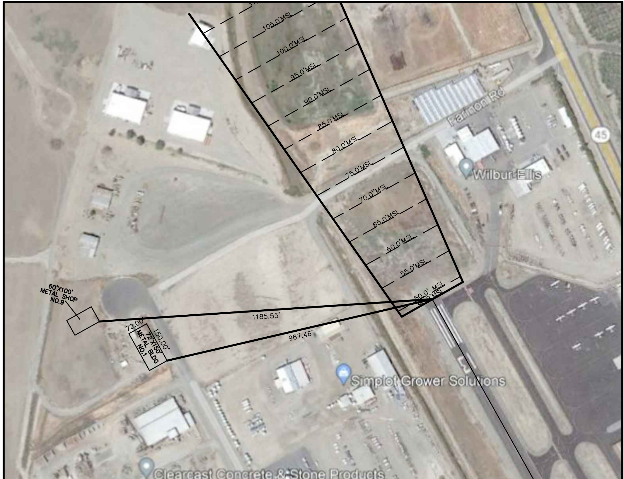
THRESHOLD SIGHTING SURFACE (20:1) 1"=200'
