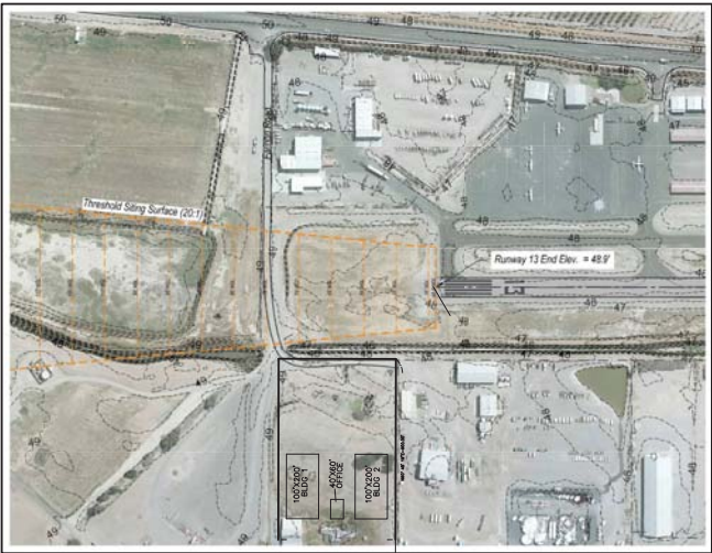
THRESHOLD SIGHTING SURFACE (20:1) 1"=200'
