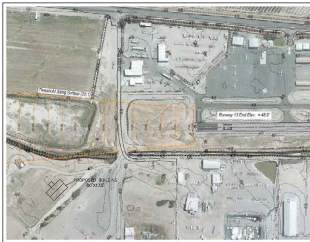
THRESHOLD SIGHTING SURFACE (20:1) 1"=200'
